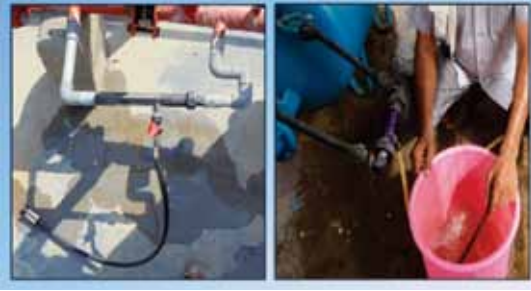
Fig. 3.4 Fertigation through Venturi
